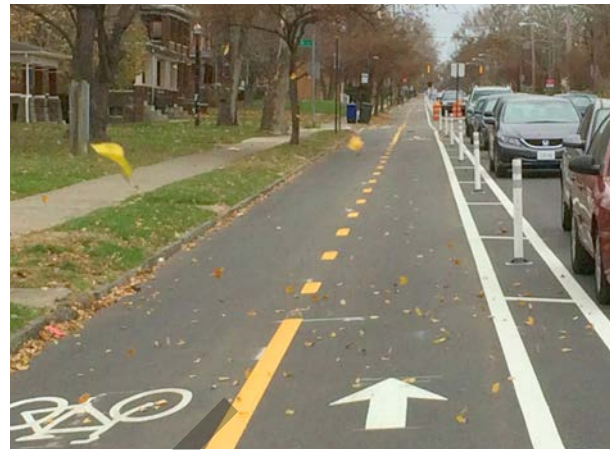
A two-way bicycle lane (shown here in Columbus), is a safe, on-road facility protected from automobile traffic by parked cars.
