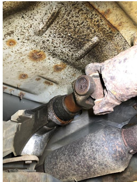
Rusted Body Mount and Floor
