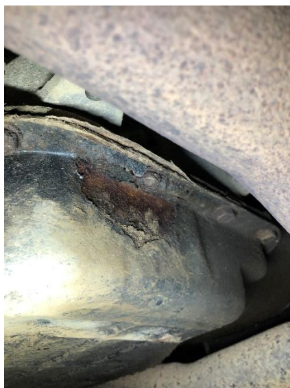
Rusted Transmission Pan
