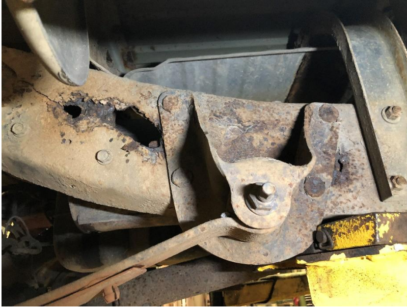
Rusted Transmission Pan
