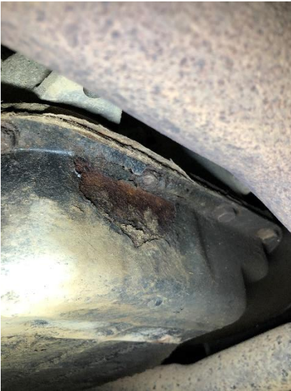
Rusted Transmission Pan
