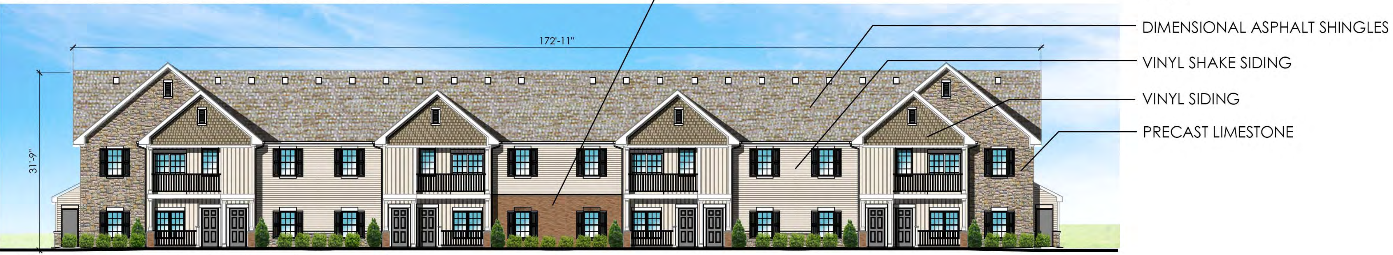
2 STORY BUILDING - 2 BED/2 BATH & REAR ELEVATION
