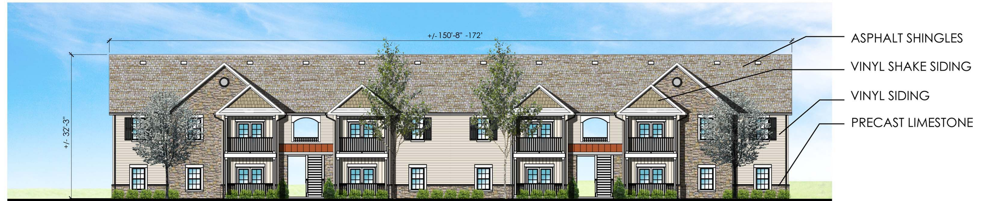
1 2 STORY BUILDING, FRONT AND REAR ELEVATION SCALE: 1"=10'
