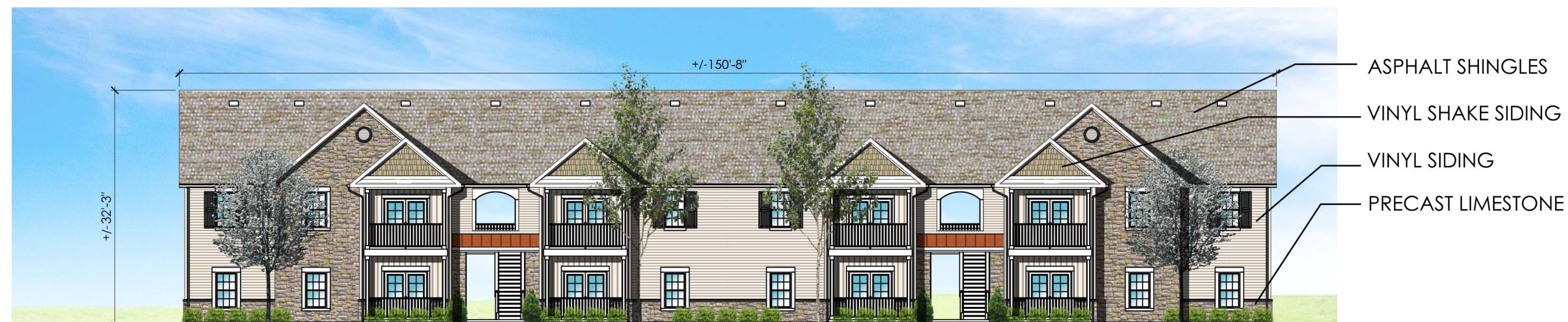
1 2 STORY BUILDING, 8 - 2 BED/2 BATH, 8 1 BED/1 BATH & FRONT ELEVATION SCALE: 1"=10'
