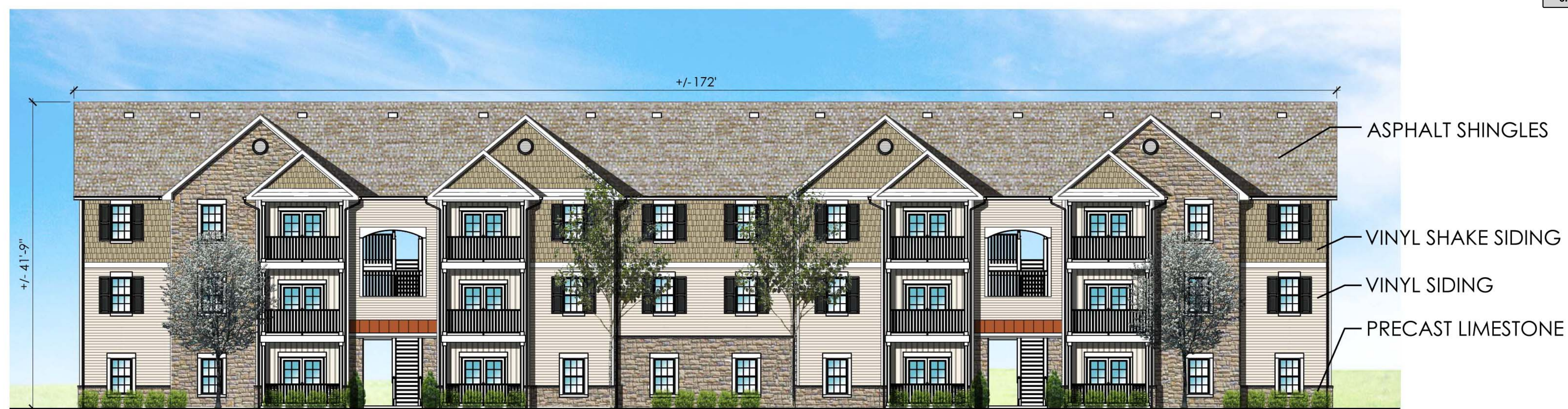
1 3 STORY BUILDING - 2 BED/2 BATH & FRONT ELEVATION SCALE: 1"=10'
