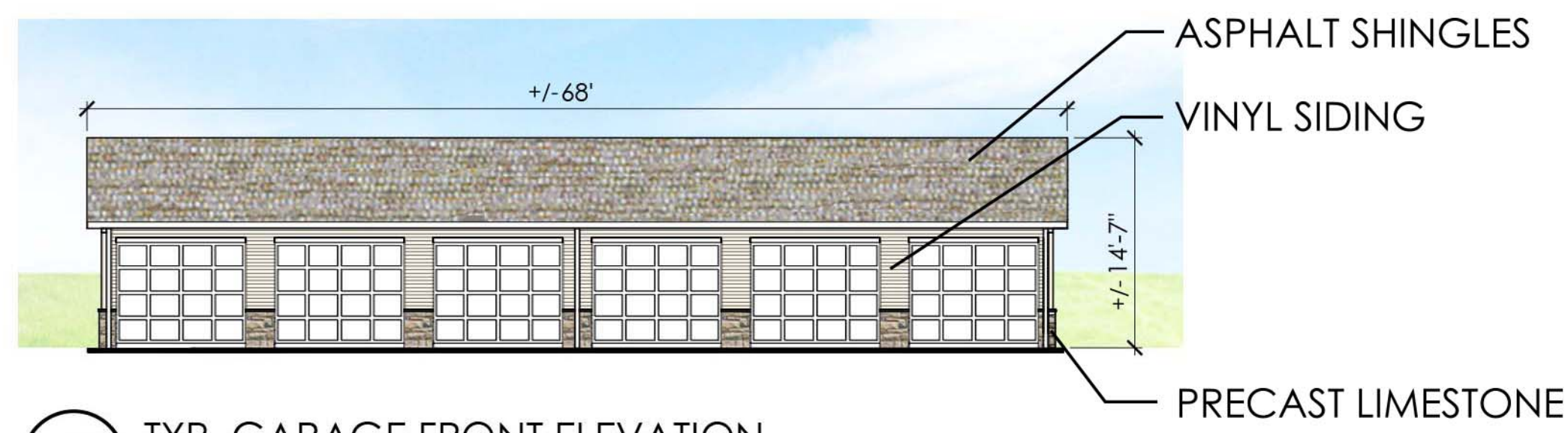
5 TYP. GARAGE FRONT ELEVATION SCALE: 1"=10'
