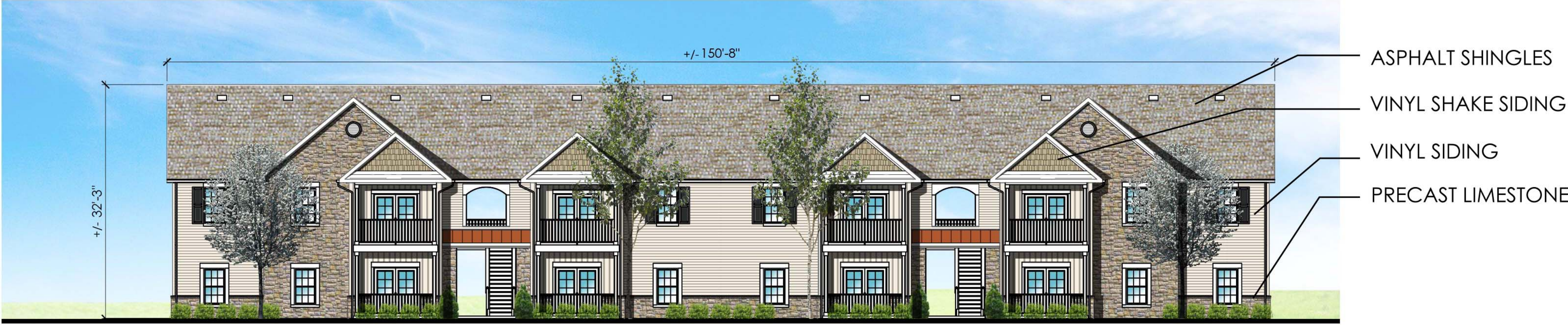
1 2 STORY BUILDING, 8 - 2 BED/2 BATH, 8 1 BED/1 BATH & FRONT ELEVATION SCALE: 1"=10'
