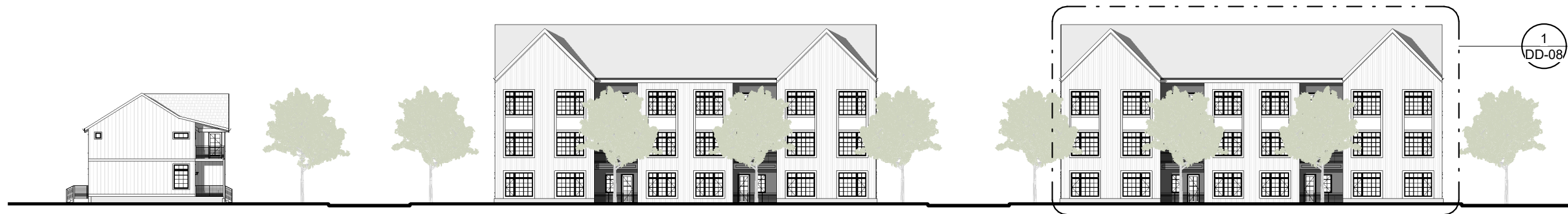
2 TOWNHOUSE & APARTMENT ELEVATION - WEST FACING SCALE: 1/32" = 1'-0"
