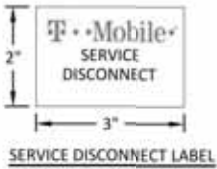
SERVICE DISCONNECT LABEL
