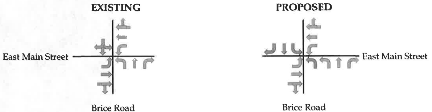
Figure 2 – Brice Road & E. Main Street Proposed Improvements
