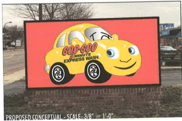
#S2-30082: FACE REPLACEMENT FOR EXISTING D/F INT. ILLUMINATED MONUMENT SIGN 3/4" = 1'-0" -FACES: PAN FORMED ACRYLIC FACES W/ YELLOW BACKGROUND AND RED & BLACK VINYL COPY.
