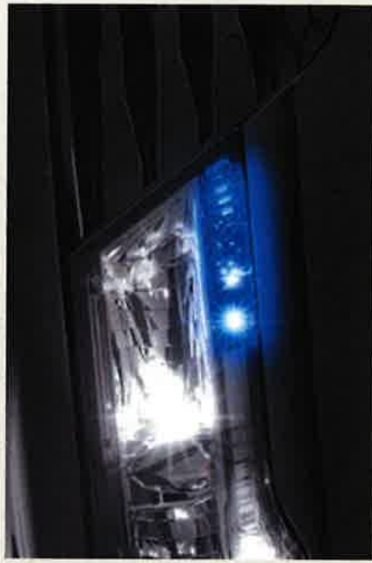
POCKET WARNING LAMPS (21W)
