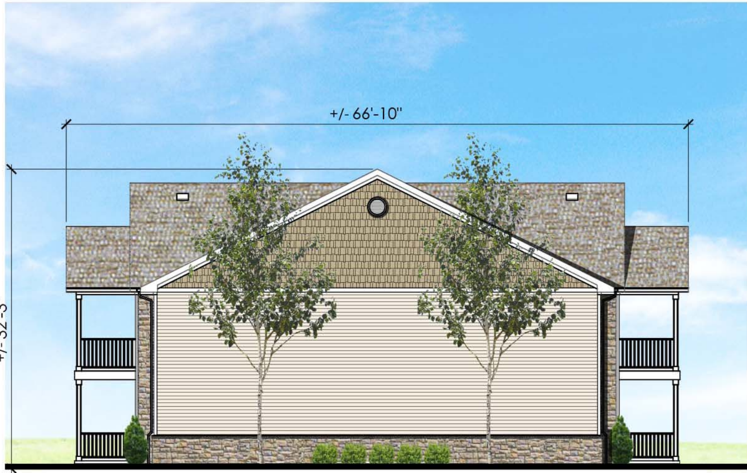
4 2 STORY BUILDING, 8 - 2 BED/2 BATH, 8 - 1BED/1 BATH & SIDE ELEVATION SCALE: 1"=10'
