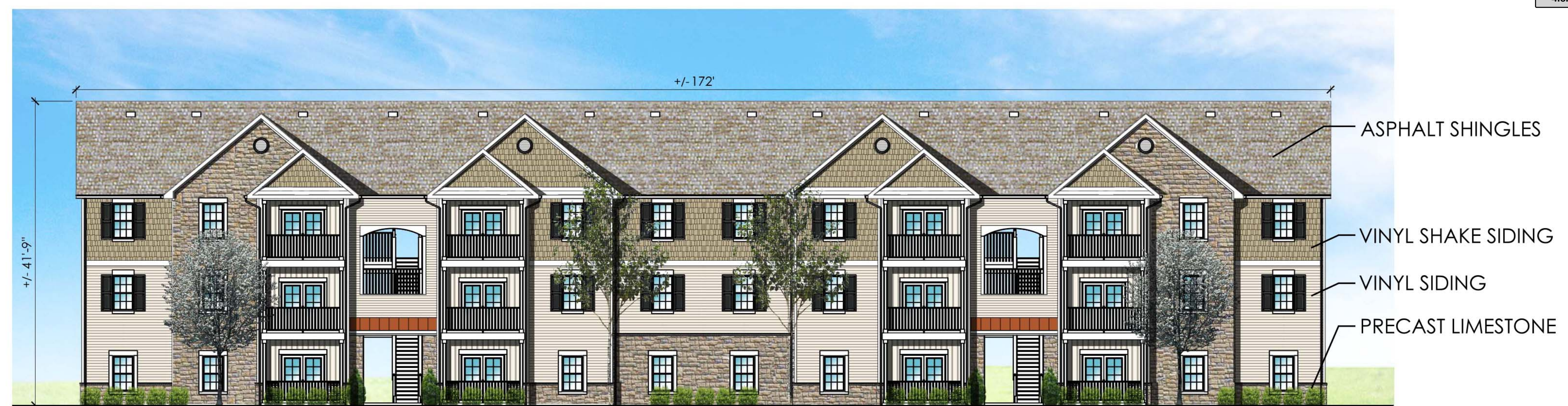
1 3 STORY BUILDING - 2 BED/2 BATH & FRONT ELEVATION SCALE: 1"=10'
