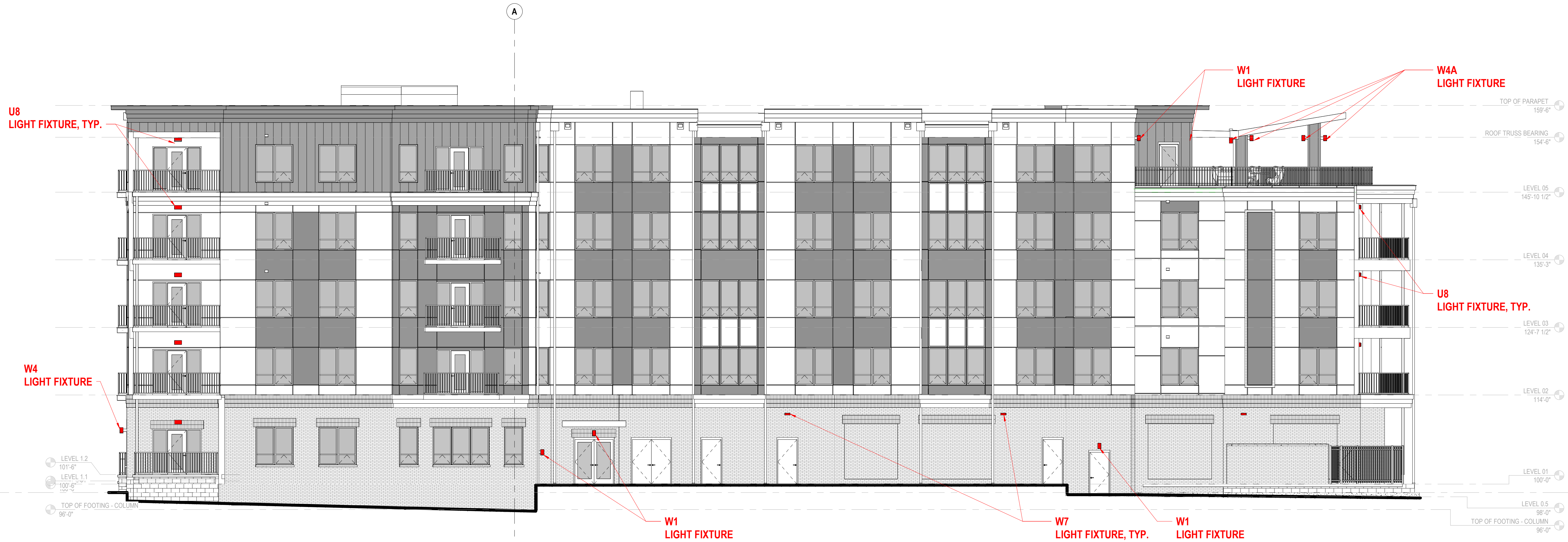
2 ELEVATION SOUTH - LIGHTING 1/8" = 1'-0"
