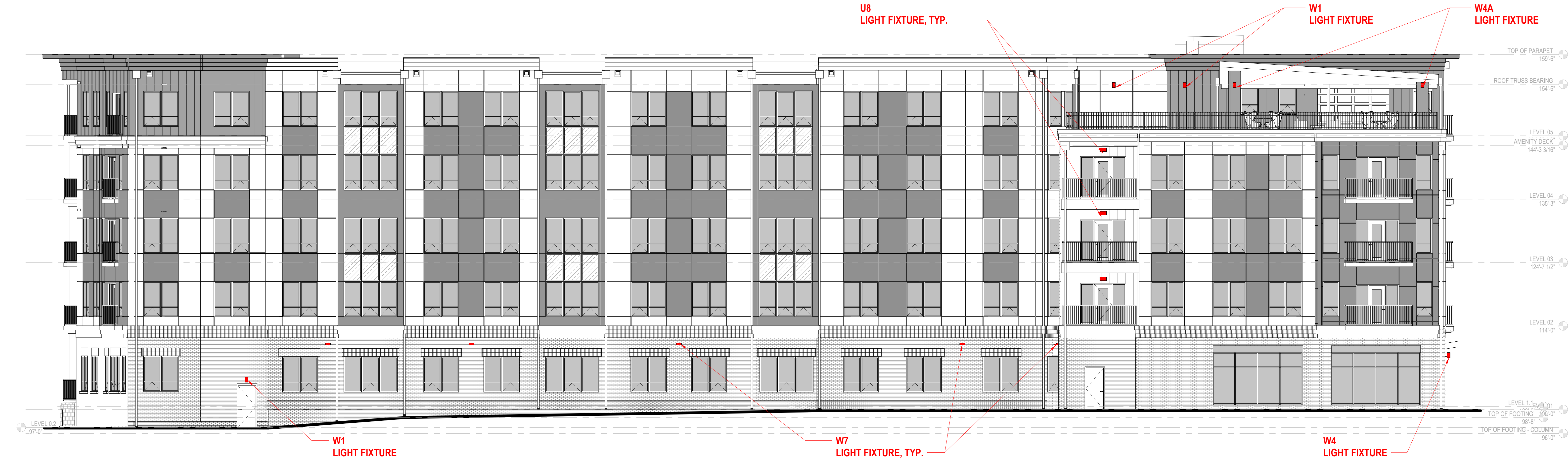
1 ELEVATION EAST - LIGHTING 1/8" = 1'-0"
